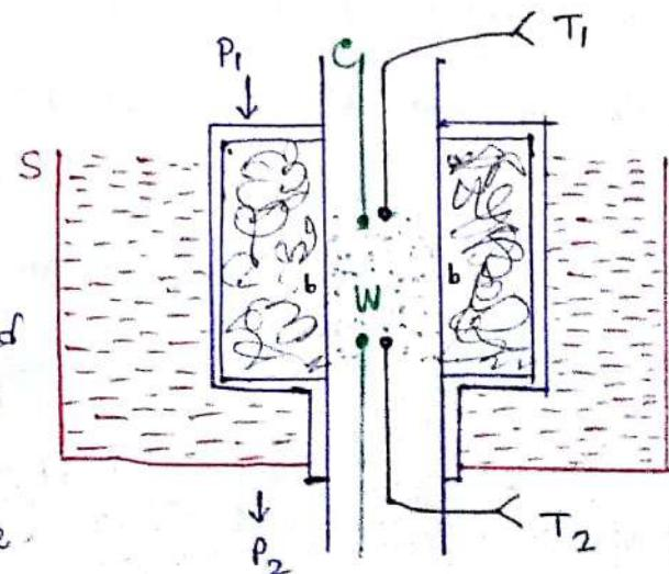
bb. The plug and part of the tube is surrounded by asbestos contained in a tin cylinder so that no heat reaches from the bath. The temperature drop is measured by the thermocouples. They worked with  $O_2$ ,  $N_2$ ,  $CO_2$  within  $4^\circ C$  &  $100^\circ C$  with initial pressure 4.5 atm & final pressure 1 atm.
