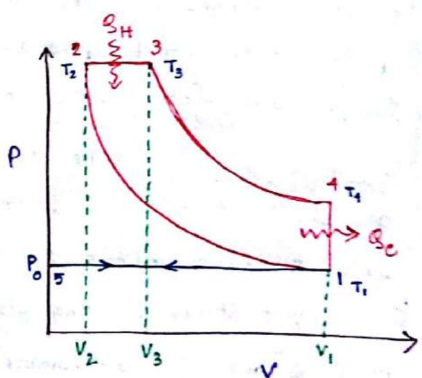
and valve exhaust releases (4→1)  $Q_c$  heat as in Otto engine,
