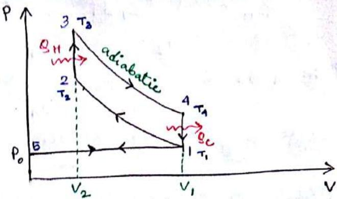
2. Compression stroke: The mixture is compressed in quasi-static adiabatic stroke until its pressure & temperature rise considerably. No friction & no loss of heat at the cylinder wall.  $1 \rightarrow 2$  process is represented as.  $T_1 V_1^{\gamma-1} = T_2 V_2^{\gamma-1}$
