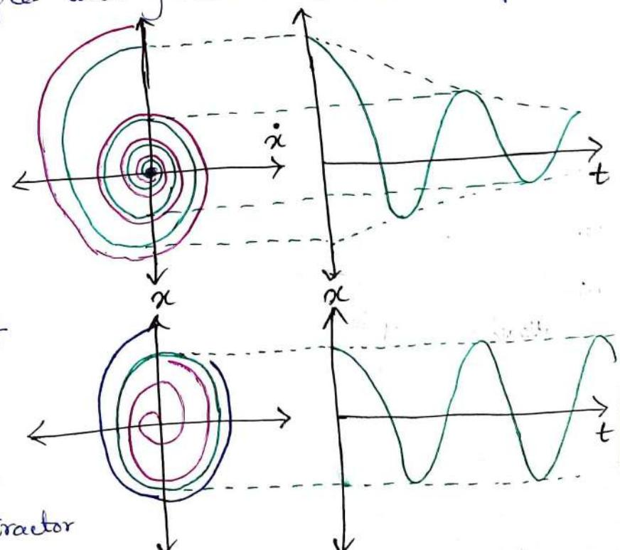
and limit cycles are the only possible attractor. The situation for nonlinear equation is different, e.g. Duffing oscillator exhibit chaotic behaviour.
