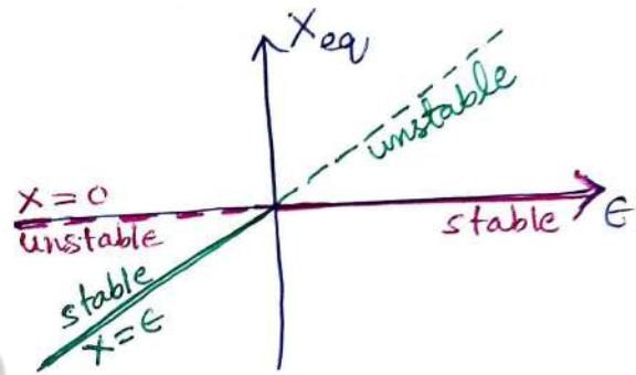
Consider the 1<sup>st</sup> order system  $\dot{x} = a + x^2$ ,  $a$  is the bifurcation parameter that is  $a=0$  and  $a \neq 0$  (both signs). for  $a > 0$ , for both signs of  $x$  no critical points exist. for  $a=0$  the system has a degenerate higher order critical point. for  $a < 0$  the system has two critical points  $x = \pm\sqrt{a}$ ,  $\sqrt{a}$  points act as a repeller and  $-\sqrt{a}$  acts as an attractor. The phase line is portrayed below.
